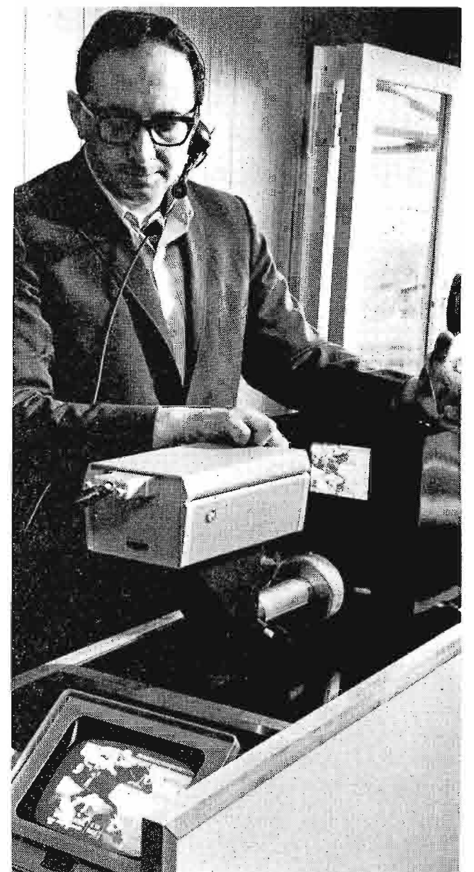
PK-302 camera focused on rear-lighted glass slide televises photo-finish pictures of race just run.
